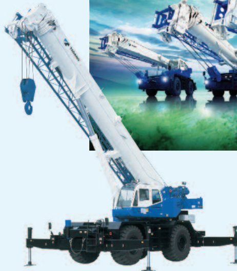
GR-600EX Lift capacity: 60t @ 3m Boom: 11.0m - 43.0m Jib: 10.1m, 17.7m
