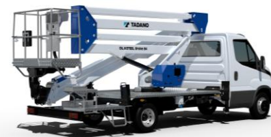
Truck-mounted AWP by PM Oil & Steel
